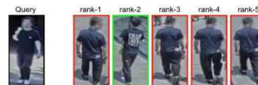
(b) Matching results filtered by direction information in addition to appearance features.
