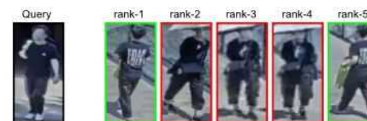
(c) Matching results filtered by time information in addition to appearance features.
